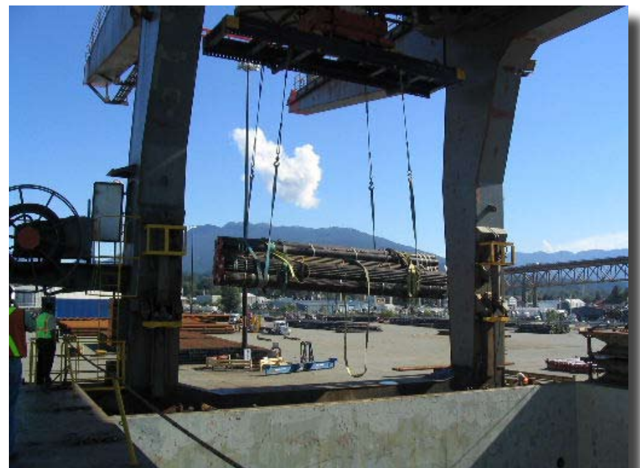
An example of double-wrapped pipe being discharged from a vessel.
