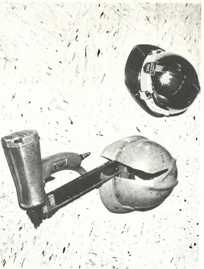
Ouch! Actually Terry Thompson of Penticton came through without a scratch when the 25 lb. staple gun shown above fell 10 feet, demolishing his hard hat. Your skull is one of the most important guardians of your brain centre. It deserves protection!
