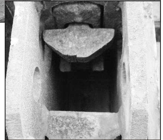
At right: Close up of twist lock in stacking flat racks.
