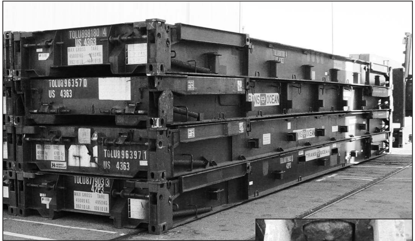
Above: Stacking collapsed flat rack containers with the built in twist locks.
